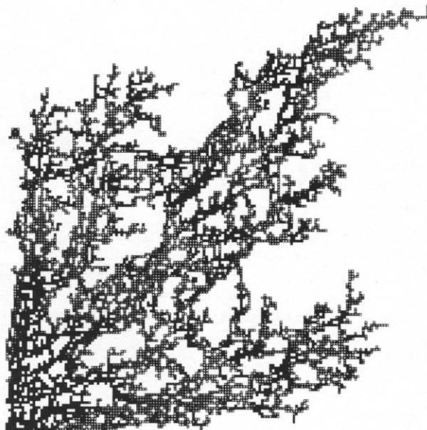
FIG. 8. The displacement front at breakthrough, using a diagonal grid, with trapped islands of the original fluid preserved. Viscosity ratio \mu_1/\mu_2 = 10^2 .
